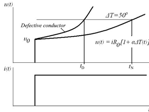
Figure 4. Plots of voltage and current load on the controlled circuit:  $t_D$  - current cutoff time in the presence of a defect in the circuit;  $t_N$  is the current cutoff time for a normal circuit when a temperature increase of  $50\text{ }^\circ\text{C}$  is reached.
