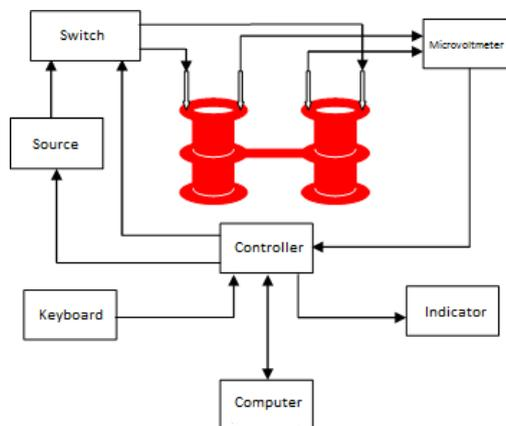
Figure 5. Functional diagram of the diagnostic stand
