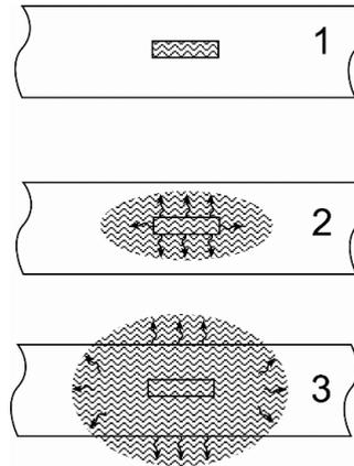
Figure 2. Stages of heating a current conductor
