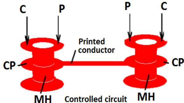
Figure 3. The scheme of connecting the probes to the controlled circuit of the printed circuit board: C and C – current probes –  $i(t)$ , P and P – potential probes –  $u(t)$ , CP – contact pads metallized holes (MH) of the printed circuit board
