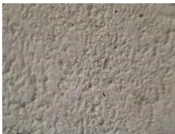
Figure 7. Microstructure of the shell surface on Armosil with 20% spirit.
