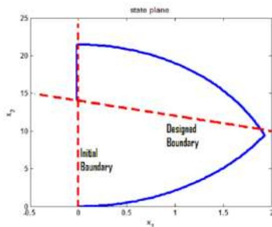
Figure 5. Diagram of state plane accompanied by inherent and designed boundary
